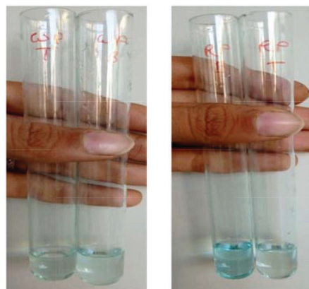
Fig. 2. Malachite green dye degradation by crude laccase enzyme
